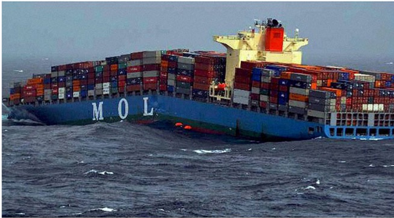
Structure and Fatigue Failure
